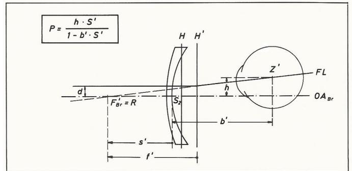
Fig. 4: Eye position behind a spectacle lens with negative vertex power when the center of rotation requirement is not fulfilled and when the fixation object lies in the direction of the optical axis of the lens.
