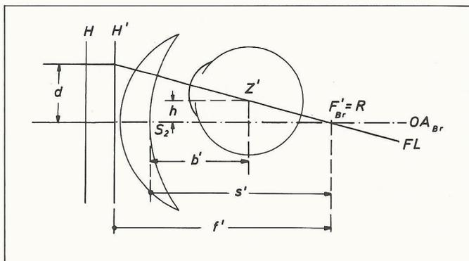
Fig. 3: Eye position behind a spectacle lens with positive vertex power when the center of rotation requirement is not fulfilled and when the fixation object lies in the direction of the optical axis of the lens.
