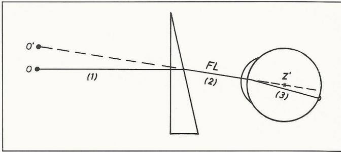
Fig. 2: Deviation of the chief ray at the visual point of a spectacle lens. O: fixated object point; O': image point produced by the spectacle lens; FL: visual axis; Z': optical ocular center of rotation; (1), (2), (3): path of the chief ray (independent of the type of lens).
